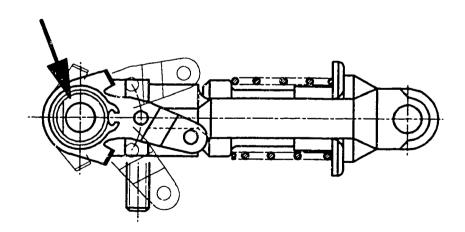
The TAS link has to be removed for testing its function. Spray the cartridge of the expansion element (1) with commercially available refrigerant spray for approximately 40 seconds until pressure disk (2) moves in direction of cartridge and comes to a standstill.
